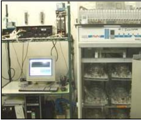
Figure 2. Equipment used to measure embryonic metabolism of individual eggs throughout the entire incubation period. A sample of air is taken from each chamber and assessed for O 2 and CO 2 concentrations. The amount of O 2 consumed and CO 2 produced by the embryo are used to calculate heat production.
